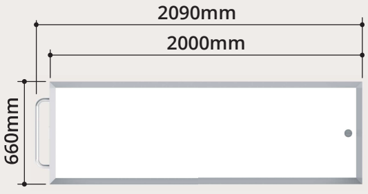
4H810P - Without drain hole H: 95mm W: 660mm L: 2090mm
